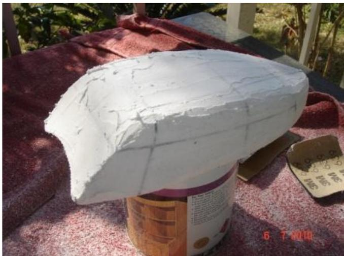
plans. I roughed out the basic shape using a big saw and 60 grit sandpaper, I can't believe how hard it is to sand this stuff, after many, many hours of sanding to get it to fit on the fuselage and look in the right proportions I smoothed it off using 100 grit paper and then iced it like a cake with lite filler.
