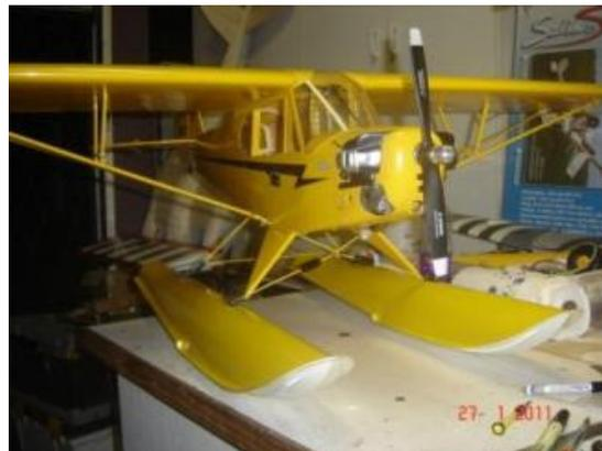
I covered the mostly desperate maiden flight on the VRCMC 'Have Your Say' page a couple of weeks ago and since then I've made a couple of adjustments to stop the severe tendency to turn left. Re aligning the RH float which Colin pointed out to me. The Cub last flew on my Futaba 6ch radio and after checking the settings the aileron right trim was set to 80%, hadn't put that into my new radio. Now all we need is some good weather and we can try a second flight.
