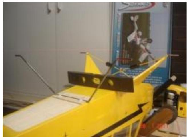
Just when I thought it was finished the rudder debate came up, don't need one, do need one, without one you can't steer on the water with just a small breeze, conclusion...fit a rudder. I bought some bits of brass, cut out a rudder shape (Ian put me right with the shape) silver soldered the bits together, bought a bendy push rod and a week or so later it was finished. Lastly I fitted a drain plug to each float, water will get in there somehow, then does it float.....
